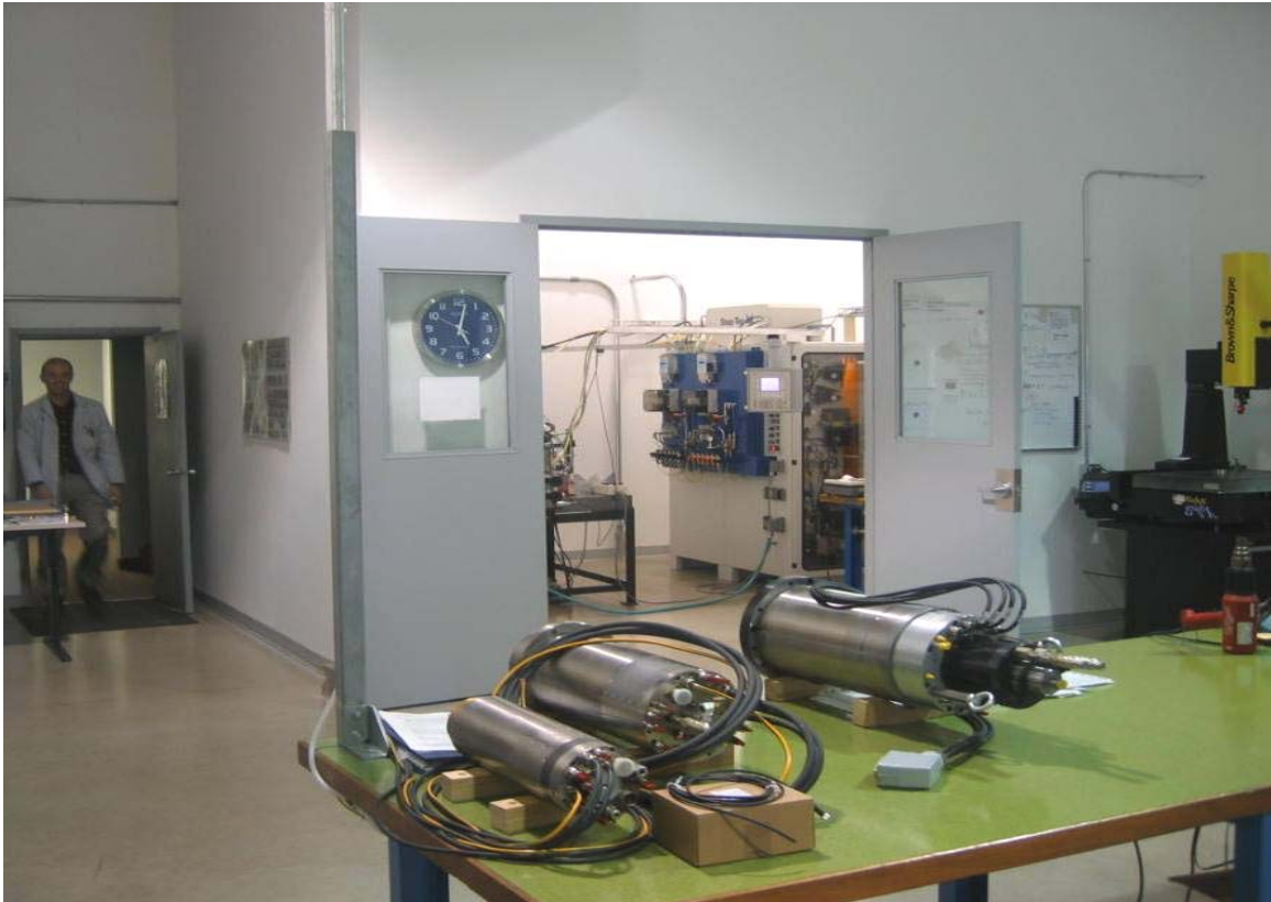
Test cell, equipped with two Siemens Universal Drives, 200 & 300 Ampere Drives, full periphery equipment to test all options on the Step Tec Spindles. Monitored via an 8 Channel Data Logger and a Simatic C7 Controller
